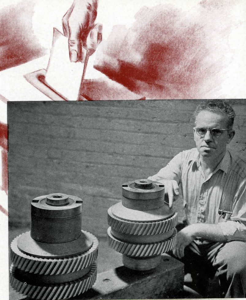
Double tool life for roto mill cutters, by reducing the diameter of three spacers, is the objective of a suggestion submitted by a "Caterpillar" Tool Inspector. The Labor-Management Committee gave an award of Exceptional Merit for this material-saving suggestion.
